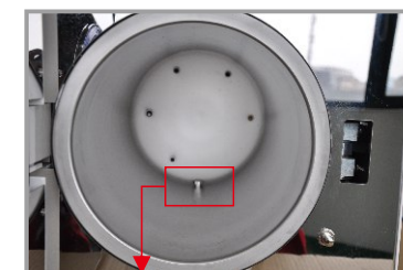
1. Chamber water filter
